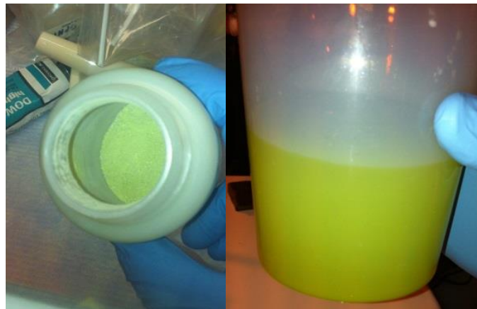
Figure 4.2 – Powdered \text{UO}_2\text{F}_2 dosed with 3wt% \text{FeF}_3 , and the powder dissolved in water
