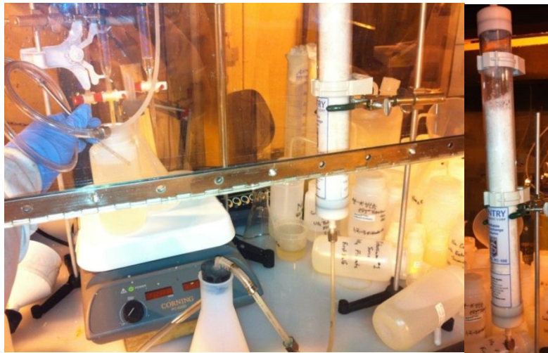
Figure 4.49 – Calcite column apparatus.
