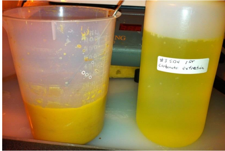
Figure 4.38 – Fifth Test Series SDU Carbonate Extraction 1. Residual solids are on the left, re-slurried in water. Carbonate extraction is on the right.
