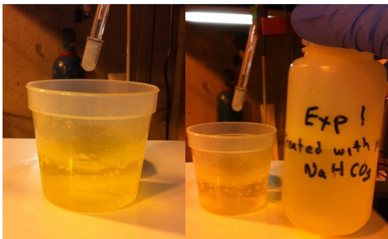
Figure 4.21 – Uranyl Carbonate Solution prepared from First Test Series SDU and \text{NaHCO}_3 , then filtered. This is the 50mL put into a small container that served as a starter solution.
